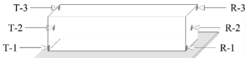
Figure 1: Schematic of UPV measurement with measurement lines indicated; T is the transmitter and R is the receiver.
